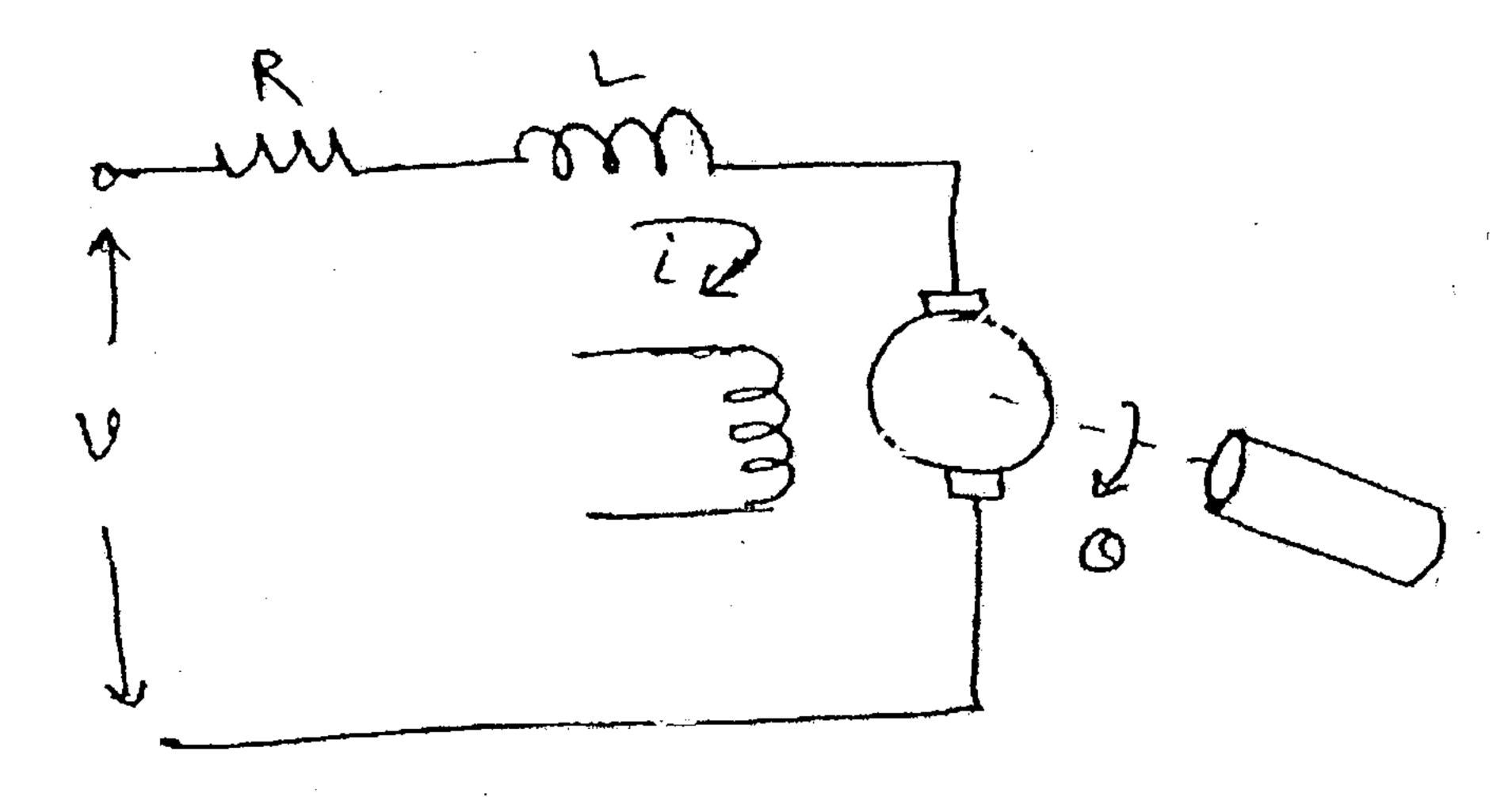
(b) Find the transfer function of the electrical network shown in figure :-
